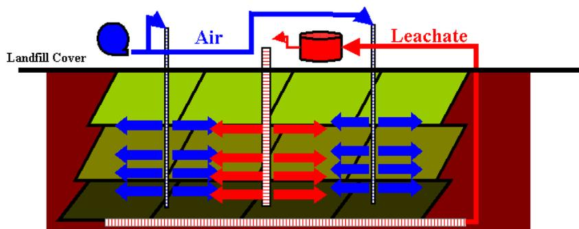
Figure 1: The Aerobic Stabilization Process at a Landfill
